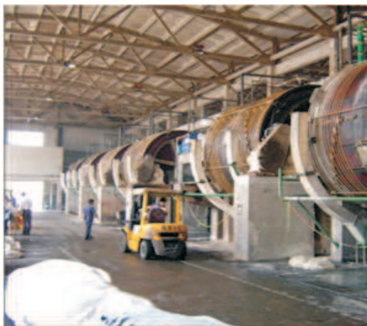
Handling with counter-balanced forklift of 3-t capacity, aisle width at least 4.8-m (about 16 feet)
